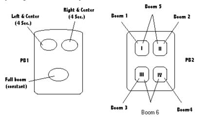
Note: If you have purchased a PB1, The upper left button will operate sections 1 & 2 for a 4 second interval. The upper right button, will operate sections 2 & 3 for a 4 second interval. The larger button on the bottom, will cause the entire boom to operate for as long as you hold the button and will shut off when you release the button.
