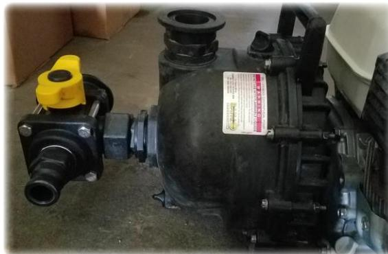
2. **Pump Outlet.** Fluid dispenses from this side when the pump is in operation.
